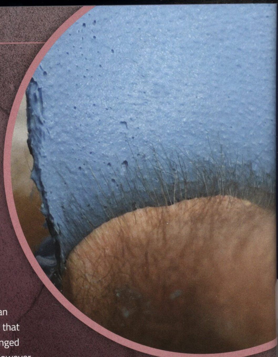
Above: Key-Form is a life casting silicone designed not to stick to hair. Here it's peeling away easily from arm hair
